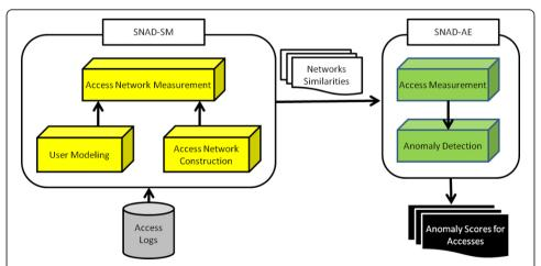
**Figure 1 The specialized network anomaly detection (SNAD) framework.** This figure depicts the architecture of SNAD. It consists of two components: 1) Similarity Measurement (SNAD-SM) and 2) Anomaly Evaluation (SNAD-AE). The SNAD-SM component constructs local access networks and measures the similarity of the users in such networks. The SNAD-AE component assesses the extent to which suppression of a user from a local access network changes its similarity.
